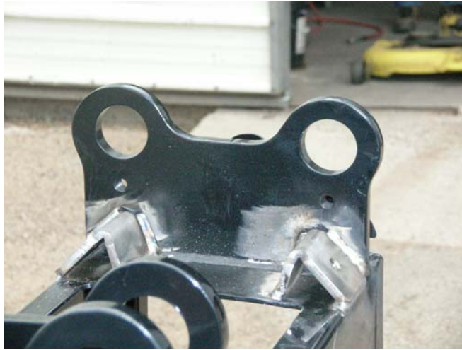
Mount brackets flush with channel.
