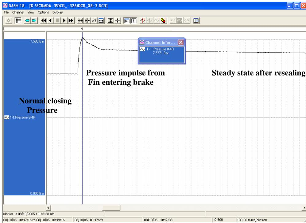
Figure 3. Chart of Pressure Pulse
